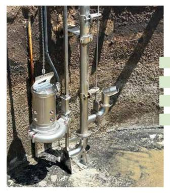
"The new Landia Chopper Pump is stainlesssteel, 30HP, with an external 5-blade knife system that continously reduces the particle size of the feedstock"
